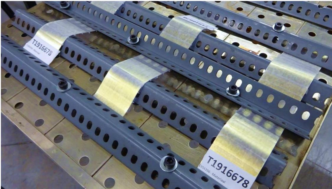
Figure 2: Clamping of the samples TOP-x5\_16mm
